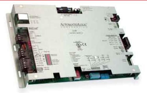
The LGR is an extremely powerful, high-speed router/gateway that can connect hundreds of control modules to a BACnet®/IP backbone. Support for BACnet/IP, BACnet-over-Ethernet, ARCNET 156 Kbps, MS/TP, and BACnet PTP communications are standard. A wide range of open and proprietary protocol translator drivers allow the LGR to also serve as a gateway to other manufacturers' equipment. Fully programmable, the LGR can also execute complex control strategies for high-level system integration.
