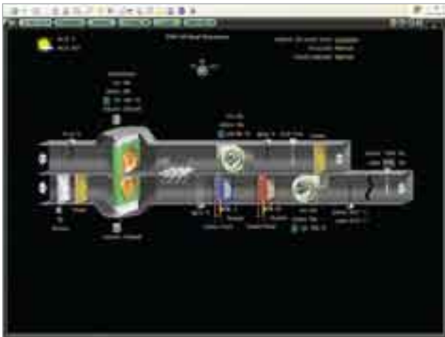
Define appropriate zone control setpoints with a simple graphical adjustment.
