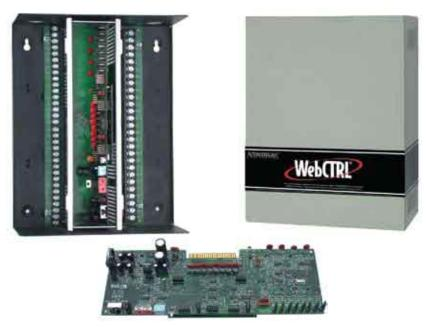
Automated Logic's WebZONE makes replacement of Barber-Colman's and Invensys's MICROZONE II controller simple! Existing control enclosures, sensors and wiring are retained, minimizing your upgrade cost.
