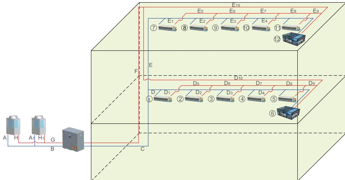
Notes: Indoor inlet is pipe 1, outlet is pipe 2 (e.g. inlet pipe number of # ① indoor unit: ① -1, outlet pipe number: ① -2)
