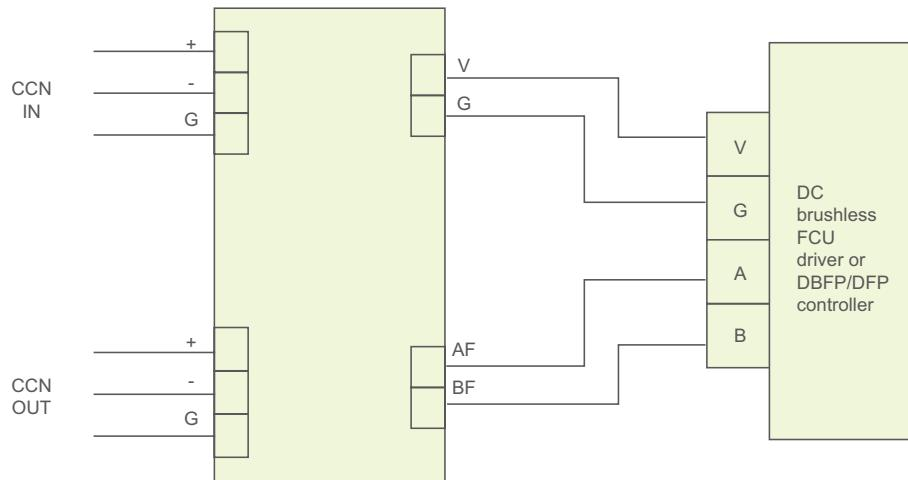
CTC200 series DC brushless FCU driver or DBFP/DFP controller wiring diagram
