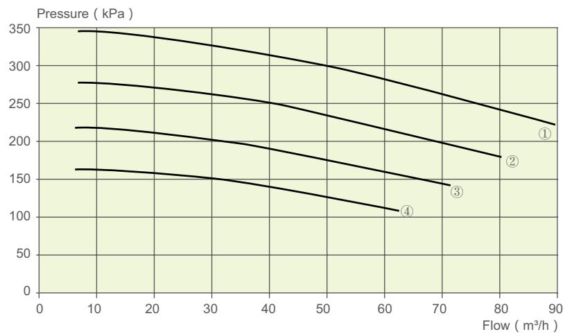
注 : ①-50Hz, ②-45Hz, ③-40Hz, ④-35Hz
