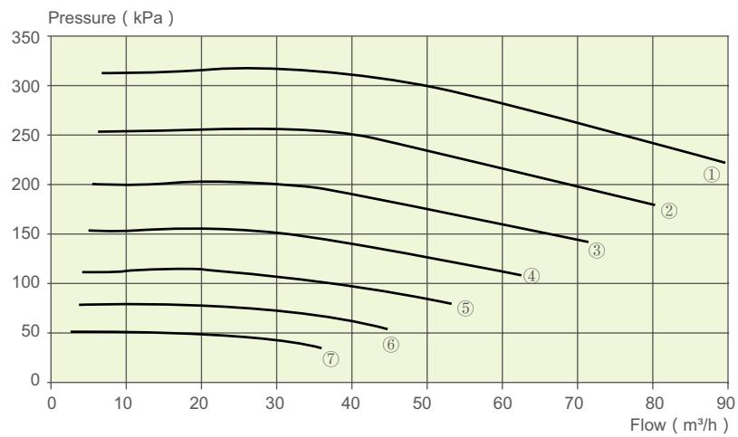
注 : ①-50Hz, ②-45Hz, ③-40Hz, ④-35Hz, ⑤-30Hz, ⑥-25Hz, ⑦-20Hz
