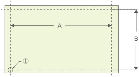
① Erection bolt4-Φ10 , threads should protrude from the supporting surface at a height less than 20mm
