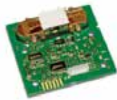
Build-in temperature and humidity sensor for return air side
