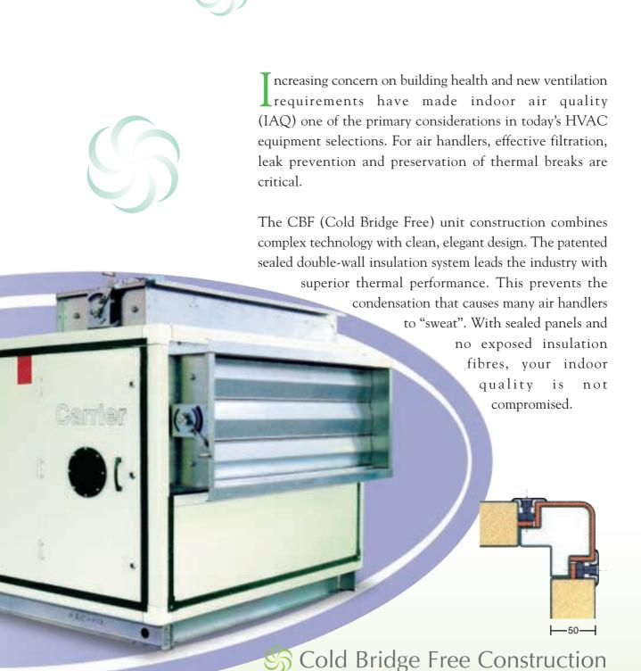
In location where the air handler is handling air with a large temperature difference between inside and outside, there is a risk of surface condensation on the inside and the outside of the unit. CBF's unique design and insulation system has eliminated the metal to metal contact between inner
