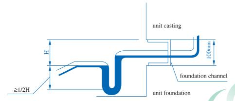
Note: H=the maximal negative pressure (mm)+50mm
